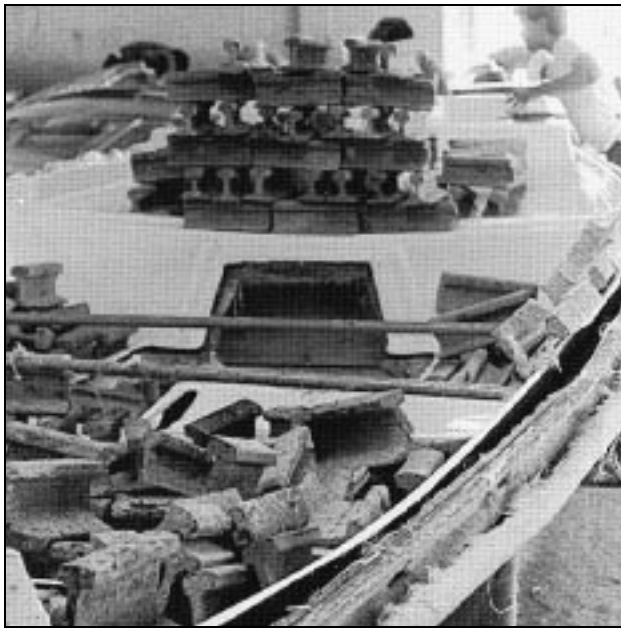
The deck molding is held in place by weights while the resin cures. The entire production process is set up to move as fast as possible, which means cutting corners everywhere.
