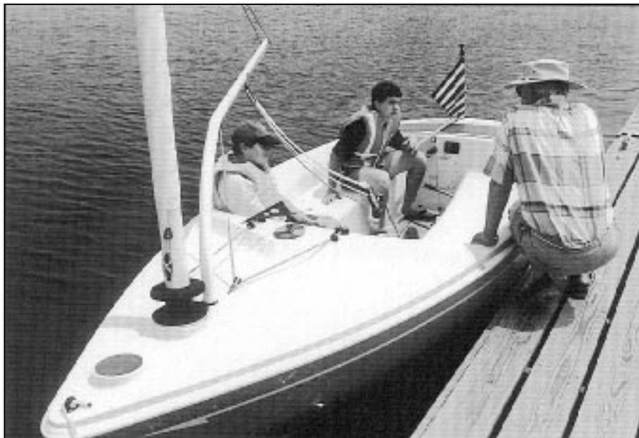
*With Garry Hoyt, the EXPO's developer, standing by, our two teenaged test pilots look over the boat's layout and controls. Note the wind vane mounted on the deck forward of the cockpit, the simple engine control handle and the big solar panel on the stern deck.*
