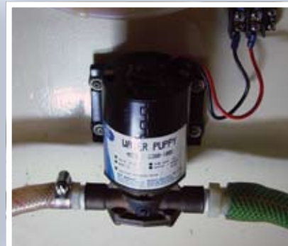
Periodic cleaning will keep your bilge pump from choking under a slurry of ick, unlike this one (above left). Regular inspection of your pump setup should include a look at fittings; notice this pump is missing a hose clamp (above right).
